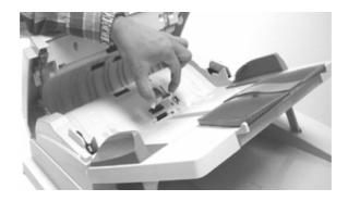
Remove the ADF pad in this direction.
